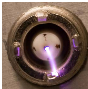
Figure 1: Photo of the 5-mm spark-like discharge in an automotive spark plug.
