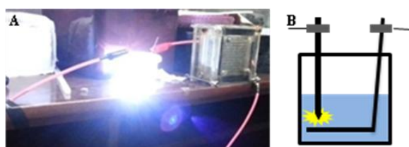
Figure 1: A. Photograph showing arc discharge, B. Schematic diagram showing arc discharge electrode.
