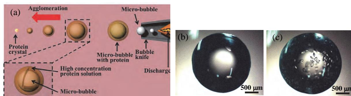
**Figure 1:** (a) *Concept of the protein crystallization assisted by electrically driven bubble knife, (b) protein crystallization by conventional hanging drop methods, (c) protein crystallization assisted with electrically driven micro-bubbles*
