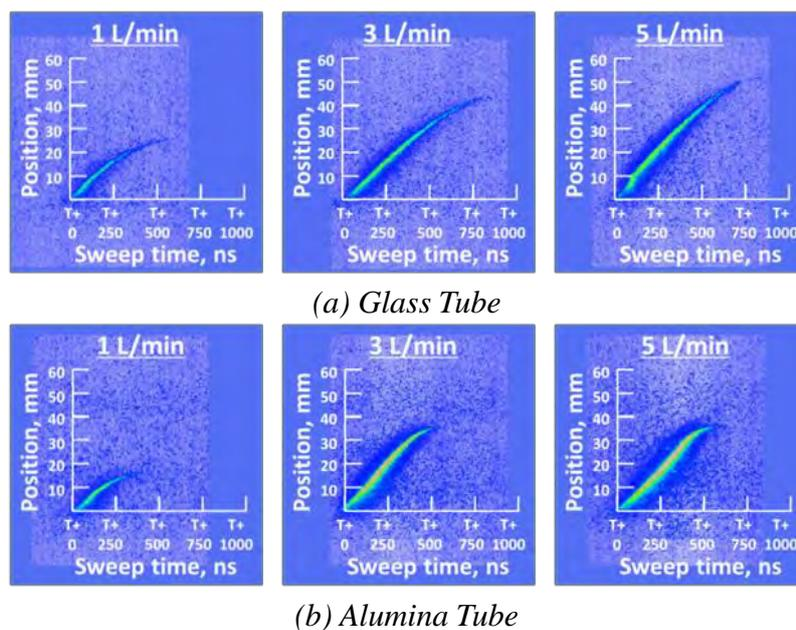
**Figure 1:** The positional dependence of the streak images of APPJs using (a) glass and (b) alumina tubes.
