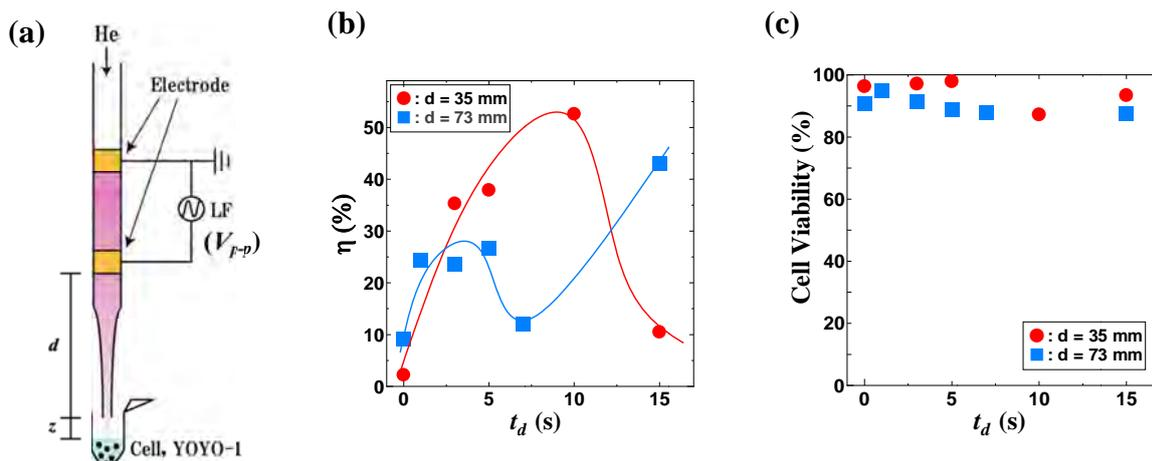
Fig. 1: (a) Schematic of an experimental setup for atmospheric pressure plasma irradiation, (b) the transfection efficiency  $\eta$  (%) and (c) cell viability (%) as a function of plasma irradiation time with the diffusion distance  $d$  as a parameter for  $V_{p-p} = 7.8$  kV,  $c = 5\mu$ M,  $z = 5$ mm.
