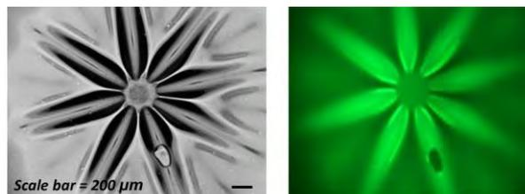
**Figure 1:** *Plasma jet treatment of the synthetic biological sensor resulting in a pattern of microchannels formed within the gelatin matrix (left bright-field image) enabling the direct plasma treatment of sensitive vesicles within the material (right fluorescence image).*
