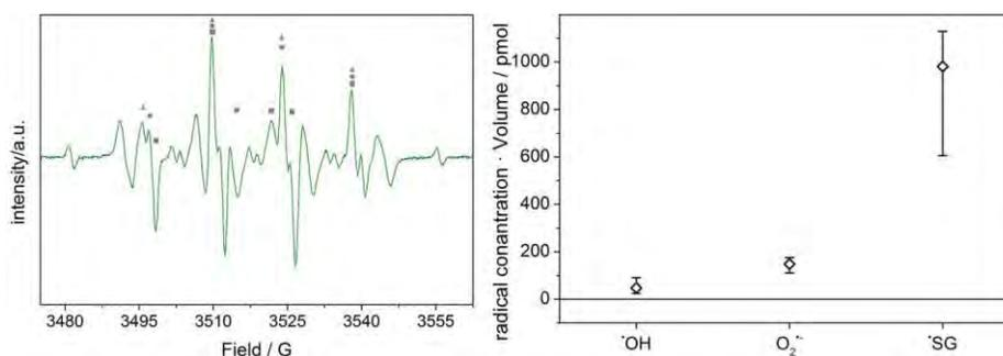
**Figure 1:** EPR spectrum after 180 s treatment with VUV radiation of an argon atmospheric pressure plasma jet and hydroxyl (marked in the spectrum with (▲)), superoxide anion (●) and glutathione thiyl (■) radical concentrations.
