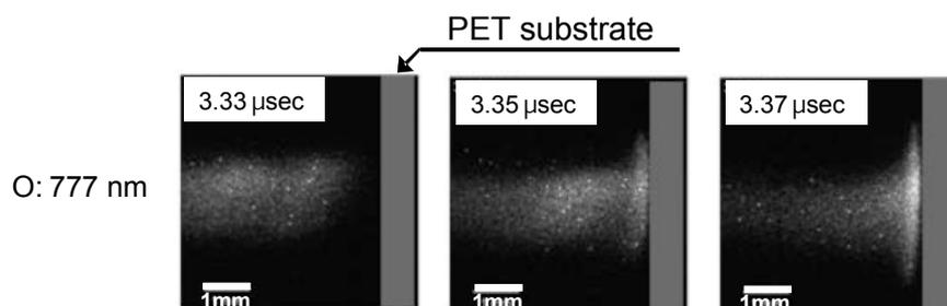
**Figure 1:** ICCD images of plasma bullet impinging on PET substrate.
