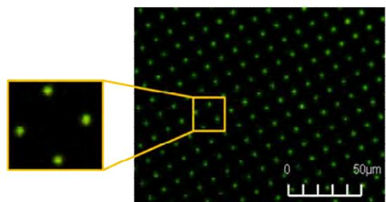
Figure 2. Fluorescent microscope image of the surface aminated dot-arrayed CNTs.
