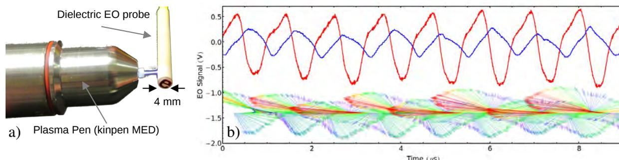
**Figure 1:** *Transient evolution of the E-field associated to the plasma jet. a) Photograph of the experiment. b) Real time measurement of the two transverse components of the E-field vector. The reconstructed E-field vectors are given below the curves.*
