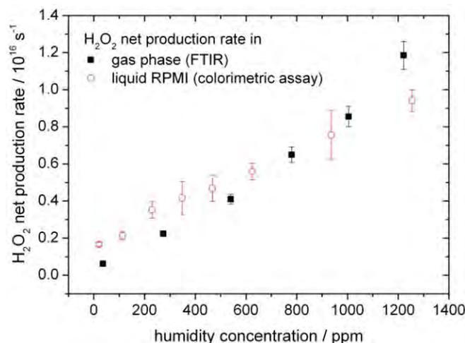
**Figure 1:** H<sub>2</sub>O<sub>2</sub> production rate is identical in the gas and in the liquid phase
