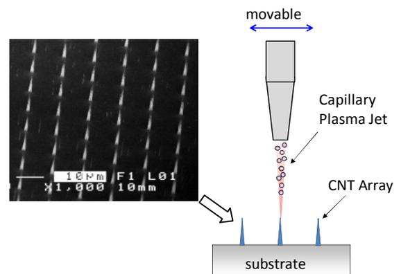
Figure 1. FE-SEM image of dot-arrayed CNTs for 1 $\mu\text{m}$  dot sizes and 10  $\mu\text{m}$  dot intervals and schematic of surface treatment
